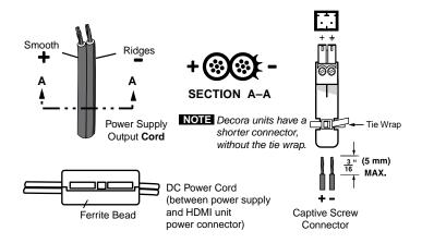
Figure 2-24 — Power connector wiring
